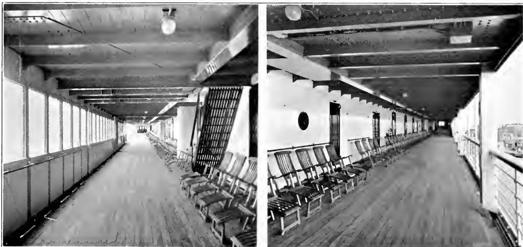
Two views of the open and enclosed promenade deck spaces on the Steamship President Hoover. Note, at right, the box girder extension of the Welin-MacLachlan gravity davits which combine the functions of a strength member in the structure of the ship and a run-way for the boat cradles.
